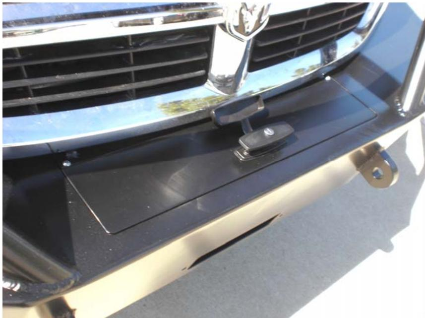
**Figure 14: Bumper door installed**
