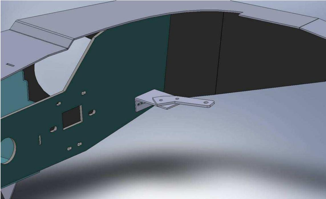
19. With the bumper hardware secured, bolt on the steel support brackets as shown in figure 9 below, using the supplied  $\frac{1}{2}$ " hardware—the slotted hole aligns with the hole in the back surface of the bumper, and the smaller hole should be against the lower surface of the side of the frame—do not tighten these bolts down fully yet, you may have to move the bracket slightly
