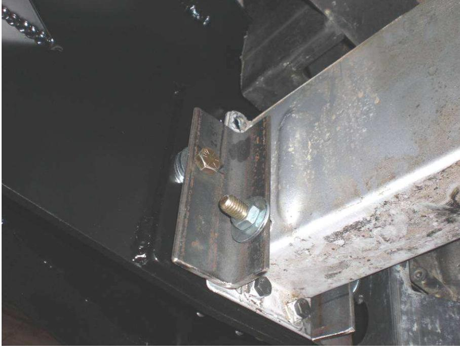
**Figure 11: Steel support brackets bolted to frame**
