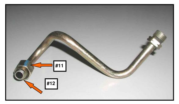
This is a picture of the factory "S" pipe that is remove during the cooler installation.
