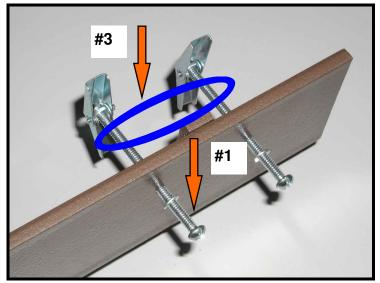
Figure #3 represents the oval in the body cross member and shows how you need to be sure the toggle screws are spread apart to the corresponding outer edges of the oval and how the toggles should be open and perpendicular to the oval opening.
