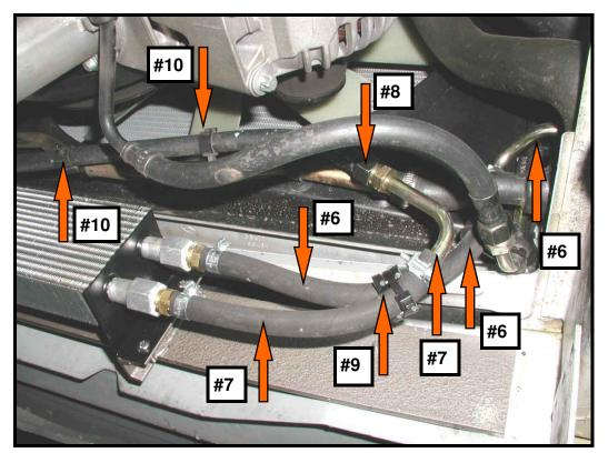
Above is a cooler installation on a 2003 Cargo Sprinter without factory rear A/C. Note the factory transmission flex hoses are routed in a slightly different position than Sprinters with factory rear A/C. Also note the cooler mounting bracket in this picture is an older version that has been discontinued.
