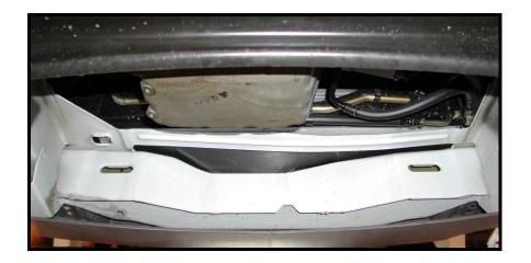
Oval mounting holes for cooler mounting bracket used in step #2 and relating to figure #3
