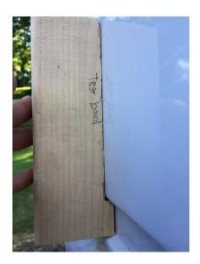
Build a test block out of wood to get the exact shape off the van for the front leading edge of the flare.
