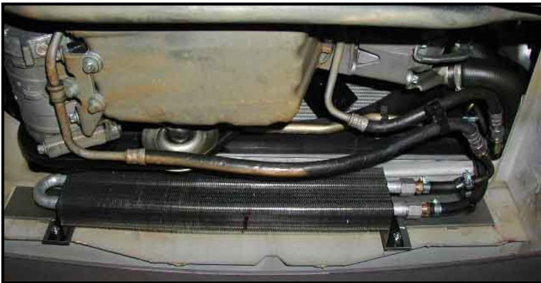
Above is a cooler installation on a 2006 Passenger Sprinter with factory rear A/C. Note the factory transmission flex hoses are routed in a slightly different position than Sprinters without factory rear A/C.
